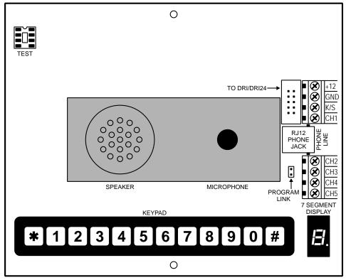
Figure 1: The DT6I with its outer cover removed.
